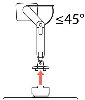
**EN** NOTE: Arm extension should be at a 45° angle or less when attaching monitor.
