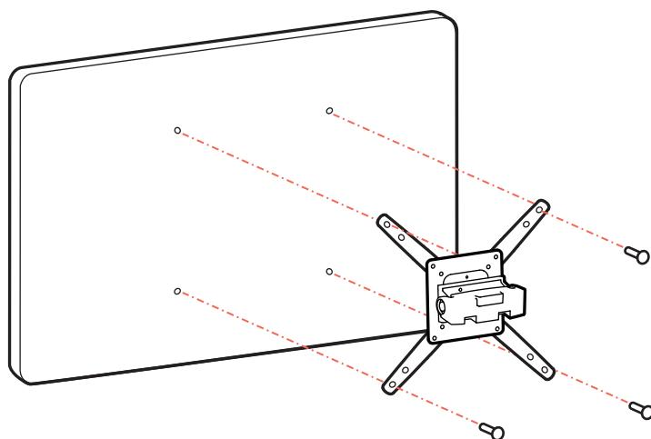
NOTE: To reduce M8 holes for use with M5 screws, or if you have a model with Samsung holder rings, follow the M8M5 KIT instructions on the next page.
