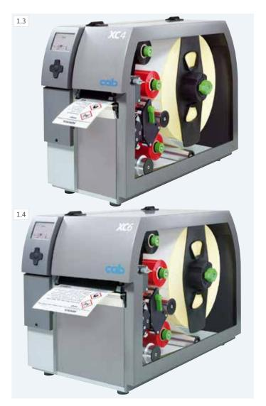
Two print units are arranged one behind the other to achieve simultaneous printing with two colors on one label.
