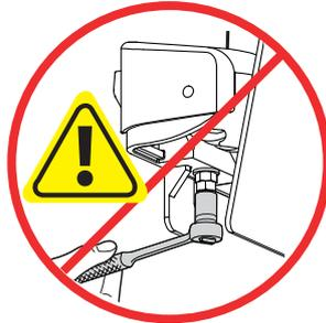
**CAUTION!** The bottom nut will turn during adjustment of the top nut; DO NOT apply any tool to the bottom nut. Serious damage to the Pivot may occur if these instructions are not followed.
