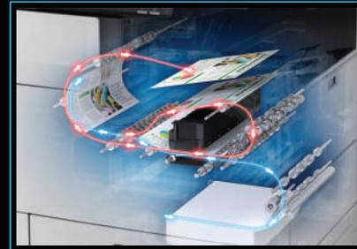
Switchback paper path design ensures ultra-fast throughput even in duplex printing.
