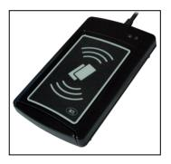
The ACR1281U-C8 is the new version of ACS's ACR120U Contactless Smart Card Reader. It is a compact and cost-effective device developed based on the 13.56 MHz contactless smart card (RFID) technology, with proximity operating distance up to 5 cm, depending on the type of contactless tag in use (supports Mifare and ISO 14443 Type A and Type B cards).
